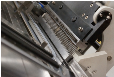
Split-punching station allowing for a punching capacity of up to 8mm books or calendars.
